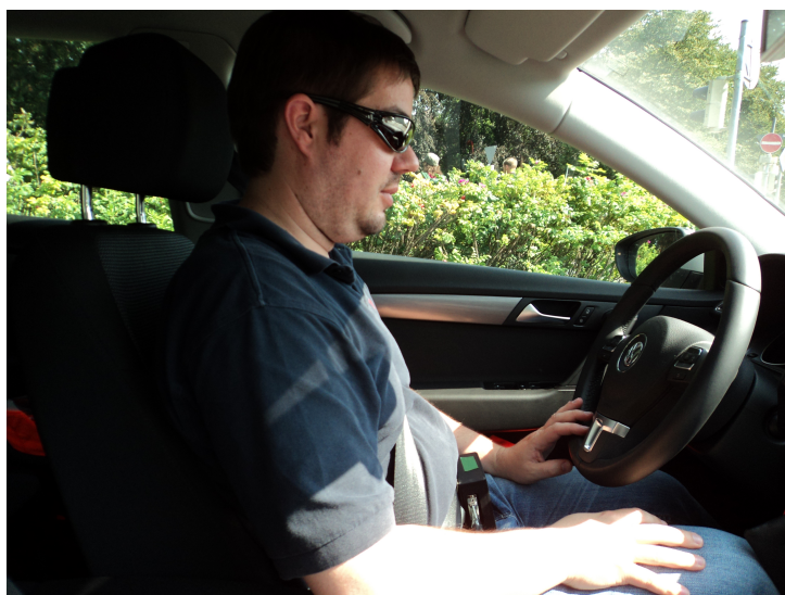
Figure 4.13: The driver wearing the tactile belt.
