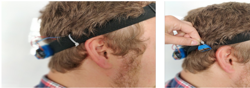
Figure 4.3: The bone-conduction speaker were placed via a headset behind the ears. [Cob19]
