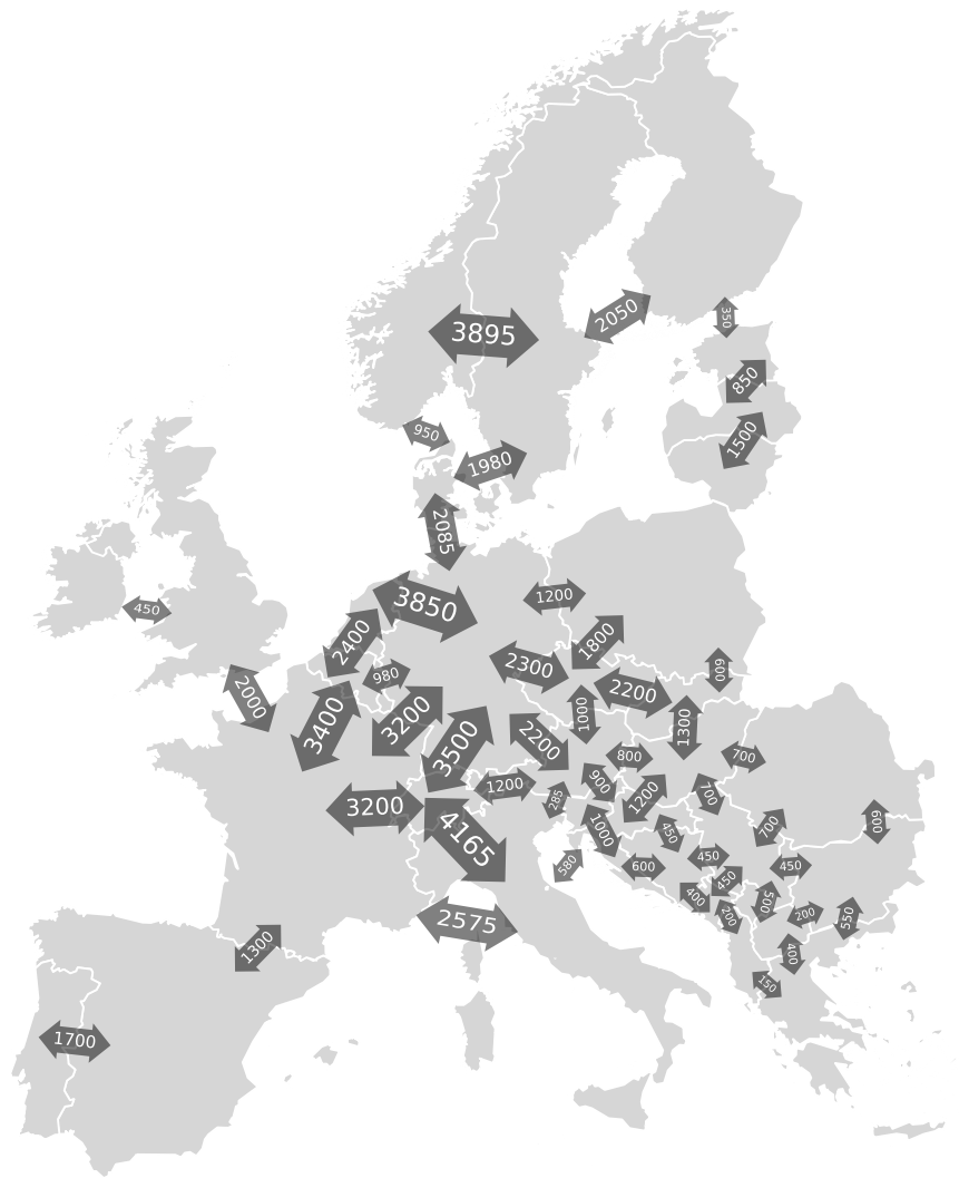
Figure 2.8: European transmission system cross-border capacities. Data bases on Entso-E (2011)
