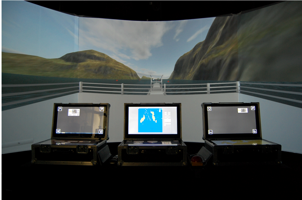
Figure 5.21: The apparatus consists of a mobile ship bridge simulator with a 202.5^\circ viewing system and three units with ship control systems, nautical instruments, and devices in an anechoic chamber. The anechoic chamber incorporated a full surround sound speaker array, with 48 speakers on the horizontal plane.
