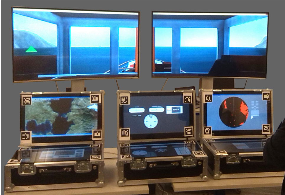
Figure 6.3: The study apparatus: A ship bridge simulator, consisting of a two display viewing system and six information displays, that were fitted with fiducial markers to mark them as AOIs for the eye tracker.
