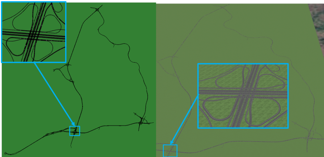
Figure 3.12: Static coupling for the highways around Frankfurt (Germany). Left side: traffic simulation. Right side: vehicle dynamics simulation [118].
