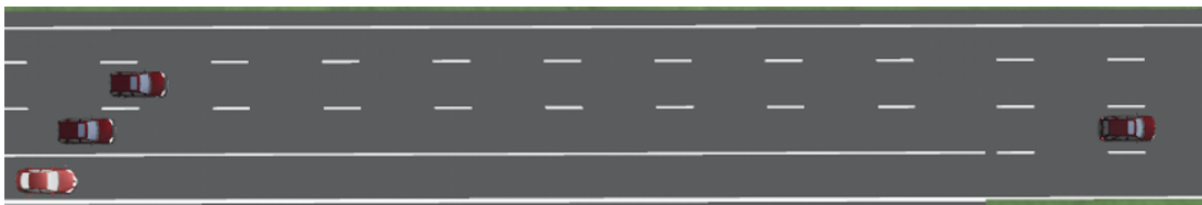
Figure 4.10: Initial conditions of the performed simulation runs. CAV colored in light red. Other test participants colored in dark scarlet [8, p. 102].
