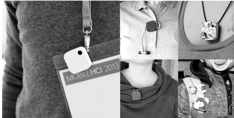
Figure 6.7: Camouflage of lifelogging cameras [Left to right, top to bottom]: unobtrusively attached to an event badge, paired with headphones to be mistaken as audio player, disguised as jewelry, worn on same-color clothing and decorated with stickers and hidden amongst buttons and pins.
