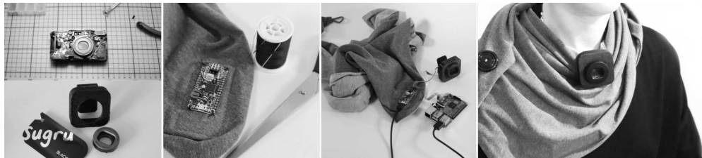
Portfolio Figure 7: Integrating custom mechanical components in form factors of the size of consumer devices is challenging. As a workaround we salvaged the iris mechanism of a discarded analogue camera, and mounted it to a 3D-printed case (left). A servo motor opens and closes the mechanical iris. As the case only fits the servo and camera lens, all other electronics, including a Raspberry Pi, and an Arduino were sewn onto a scarf (middle) or worn hidden under it (right).
