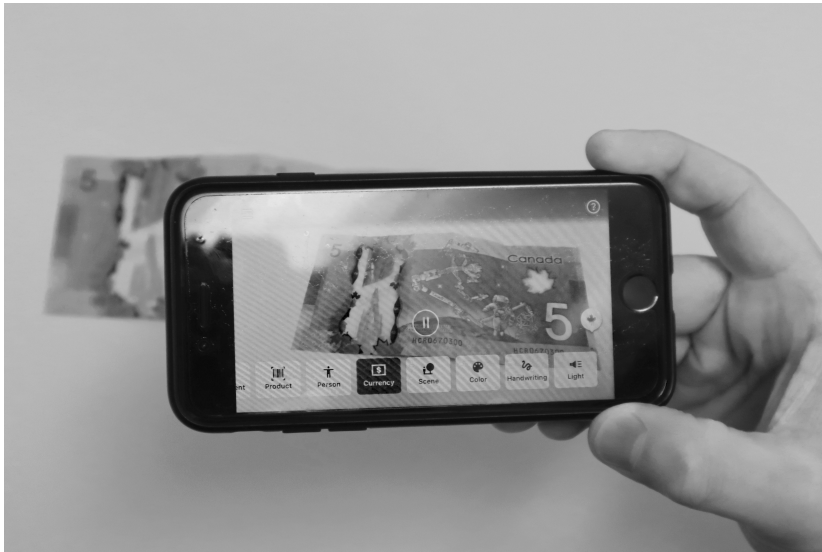
(a) The banknote's value is visually detected, and provided to the user as audio output: "Five Canadian Dollars".
