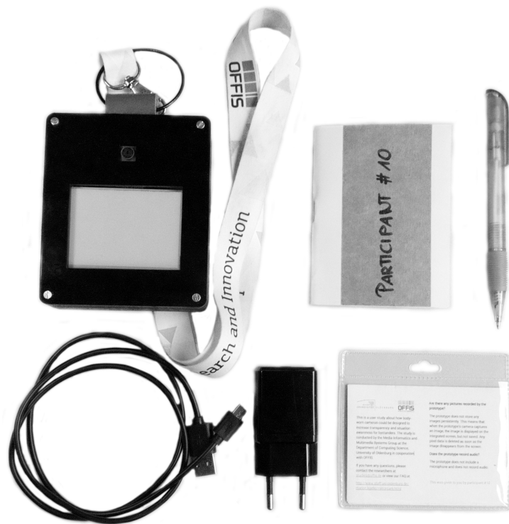
Figure 6.5: Study equipment, including MirrorCam prototype, charger, an A7 journal (“diary”), and a set of information cards.
