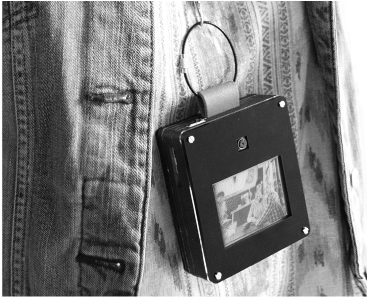
Figure 6.2: The MirrorCam prototype is a chest-worn camera including a screen-based status indicator. We contribute our experiences from an in-the-wild study where participants tested the prototype in their everyday lives and collected 79 hypersubjective impressions in their pen-and-paper diaries.
