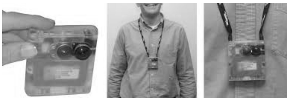
Figure 1.4: Early prototype of the SenseCam [SFA + 07]. Body-worn cameras have been successfully used as research vehicles: originally envisioned and prototyped by Lyndsay Williams as wearable accident recorder, the SenseCam became part of a dissemination initiative initiated by Steve Hodges that promoted the device for various research applications. According to Microsoft 3 the SenseCam was used in the creation of over 200 research papers.
