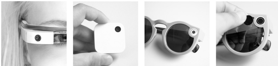
Figure 4.11: For bystanders it is not always easy to determine whether state-of-the-art body-worn cameras are recording them: some devices, such as Google Glass Explorer Edition (left) or the Narrative Clip (2nd from the left) do not provide any status indicator or privacy notice. Other devices, e.g., Snap’s Spectacles (2nd from the right), provide LED indicators. However, those can be easily overlooked, misunderstood, or hidden, e.g., by applying stickers (right).
