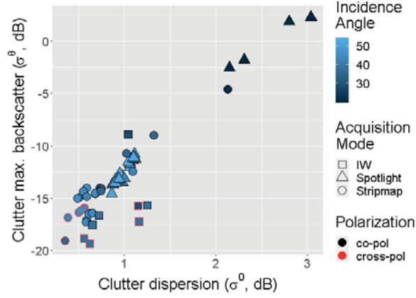
Figure 4.15: The water surface’s maximum backscatter and dispersion and its relation to different sensor parameters.
