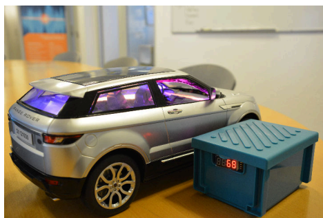
(b) The sensorbox next to the prototype displaying the currently measured distance.
