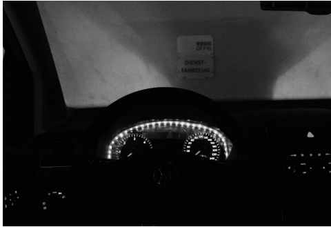
(a) An LED strip with a simple pattern to demonstrate a possible location or a pattern of an ALD (see Section 4.1).
