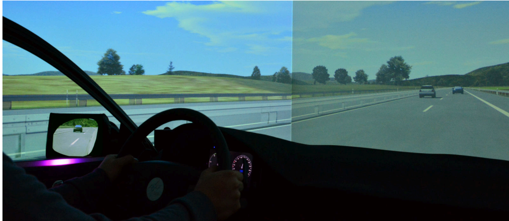
Figure 5.10: Our driving simulator during the experiment. The purple light gives information about the distance to an approaching rear car on the target lane via its location and brightness. In front is a slower car on the same lane and a faster car on the left lane. The driver now has to decide if he or she wants to overtake.
