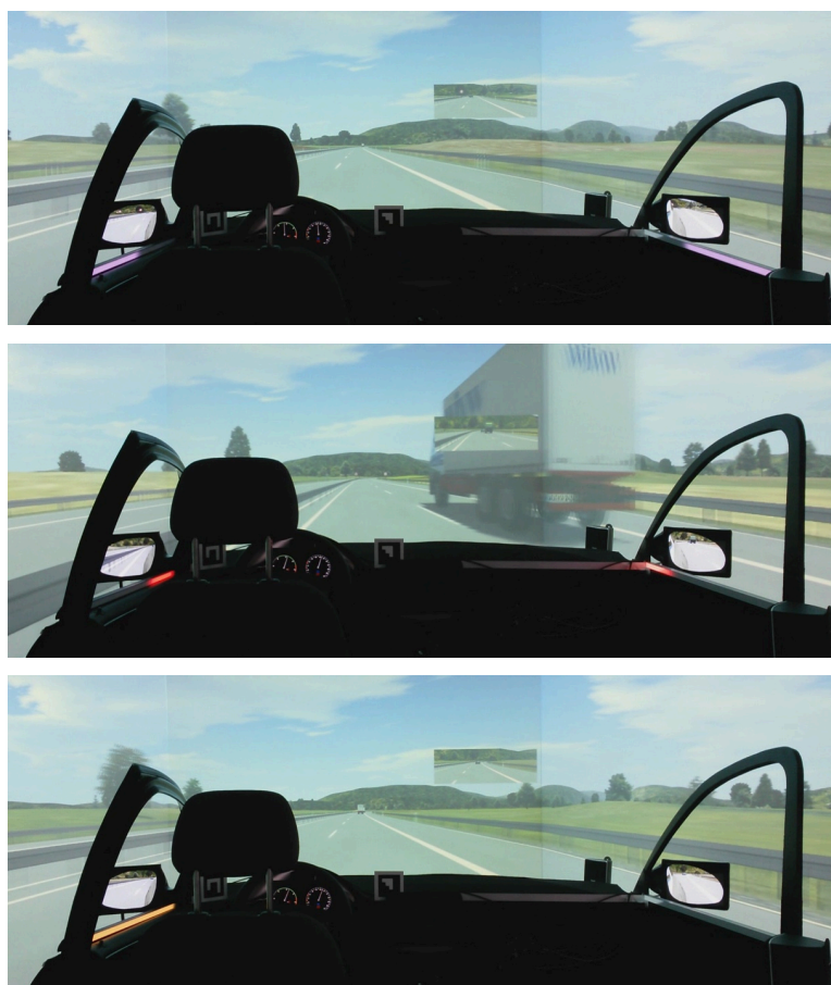
Figure 6.10: The implemented light pattern, embedded in the driving simulator. From top to bottom: accelerating, braking, changing lanes to the left.
