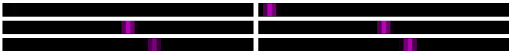
Figure 5.11: Example states of both light patterns. Left: Adapting light pattern; Right: Constant light pattern. First row: TTC = 19s , distance_{rear} = 95m ; second row: TTC = 10.8s , distance_{rear} = 54m ; third row: TTC = 9s , distance_{rear} = 45m . In contrast to the constant pattern, the brightness of the adapting pattern is highest around 54m and decreases to both ends.
