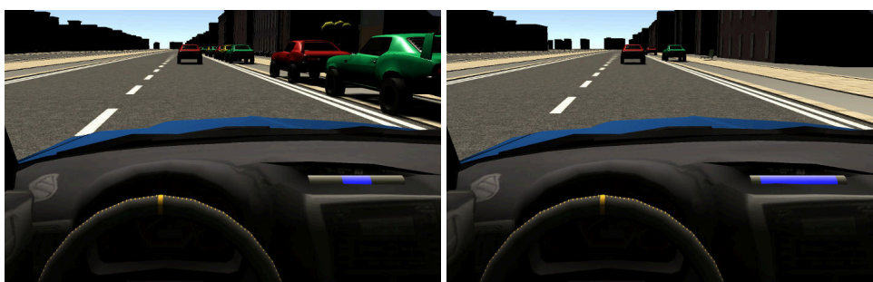
Figure 6.8: ALD pattern above the central console for “no parking space”. Left: few available slots, right: many free parking spaces.
