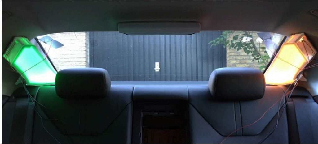
Figure 4.9: Our integrated prototype with light displays at the C-pillars. Left: green (1.5m-2.5m), right: orange (0.5-1.5m).
