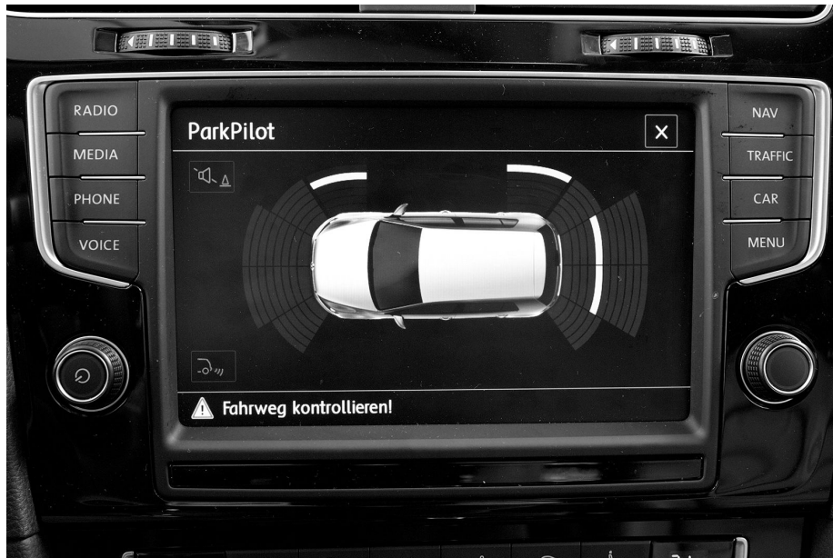
Figure 4.6: An example of a park distance control system from VW. By Nozilla ( https://commons.wikimedia.org/wiki/File:Parking_Assist.jpg ), "Parking Assist", https://creativecommons.org/licenses/by-sa/3.0/legalcode .
