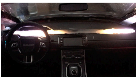
(f) An example light pattern: two dynamic lines of light approaching from either side of the LED strip attached inside the dashboard.
