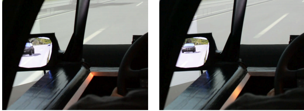
(a) Discrete pattern with fixed light in the front left corner. (b) Continuous pattern with moving light along the left side.
