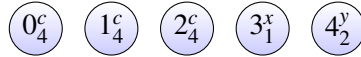
Figure 1.3: Five replicas after writing the value c with VN 4 to the replicas 0, 1, and 2.
