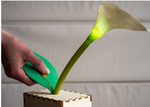
Figure 3.10: The Social Flower presenting a high activity-level with a green light color. A user touches the leaf of the Social Flower to send a greeting to a connected loved one.
