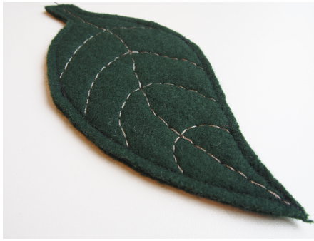
Figure 3.12: Leaf made from soft fabric and conductive thread to enable touch-input.
