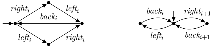
Figure 11.3.: A model of a single philosopher (left) and a model of a single fork (right).
