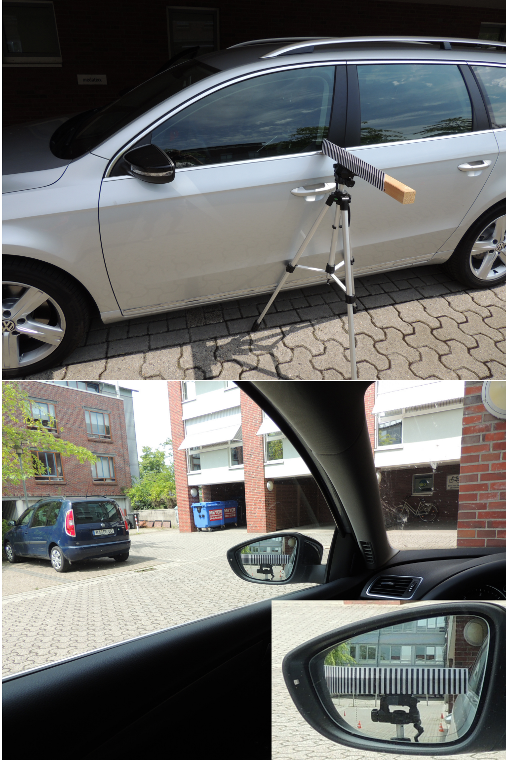
Figure 7.10: Top : Positioning of the reference object in 75 cm distance to the mirror. The height was adjusted to equal the center of the mirror. Bottom : The photo taken from the drivers perspective from the exact same position as in Figure 7.9
