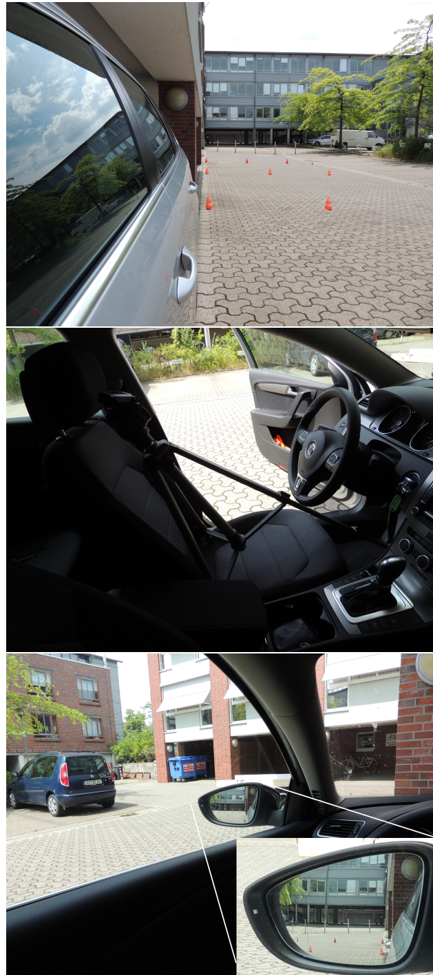
Figure 7.9: Top : Positioning of the test vehicle. The pylons are located in 5m distances backwards and 2m distances sideways Middle : Positioning of the camera in the test vehicle. Bottom : The mirror was adjusted horizontally until the first row of the pylons just disappeared from the bottom of the mirror.
